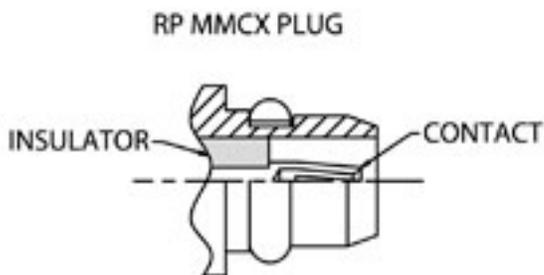
MMCX Reverse MMCX plugs have the dielectric and center socket of the MMCX jack inside the MMCX body. To identify them, look closely into the center of the connector. If you find a socket contact in a body with external snap-ring, you have an RP MMCX plug. They will not mate with standard MMCX jacks. To attempt to do so will damage contacts in both connectors. All performance and function characteristics of the MMCX connector apply to the RP MMCX.
