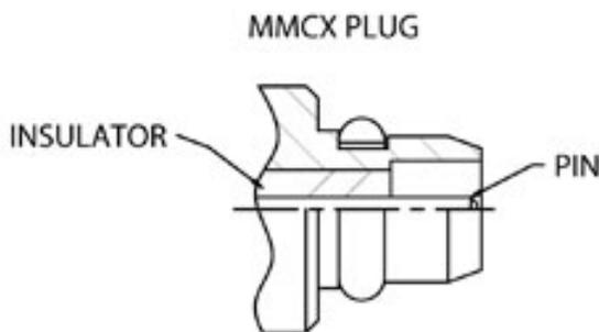
The MMCX, "miniature MCX", micro-miniature series of 50Ω connectors was developed in the 1990's for use with densely packed PCB layouts. They are about half the size of the SMB. Their lock-snap coupling mechanism with non-slotted outer contact allows 360 degree rotation without loss of broadband performance and with low reflection from DC to 6 GHz. MMCX connectors conform to European
